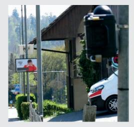
PeCo NoiseTraffic is the directional detection of the noise of moving vehicles. Here, PeCo NoiseTraffic distinguishes between vehicle and ambient noise. At the same time, traffic is counted according to direction. The distinction between the vehicle classes motorcycle - car - truck - bicycle also provides information about the road users (developments to differentiate between electric cars and electric bicycles in preparation).
